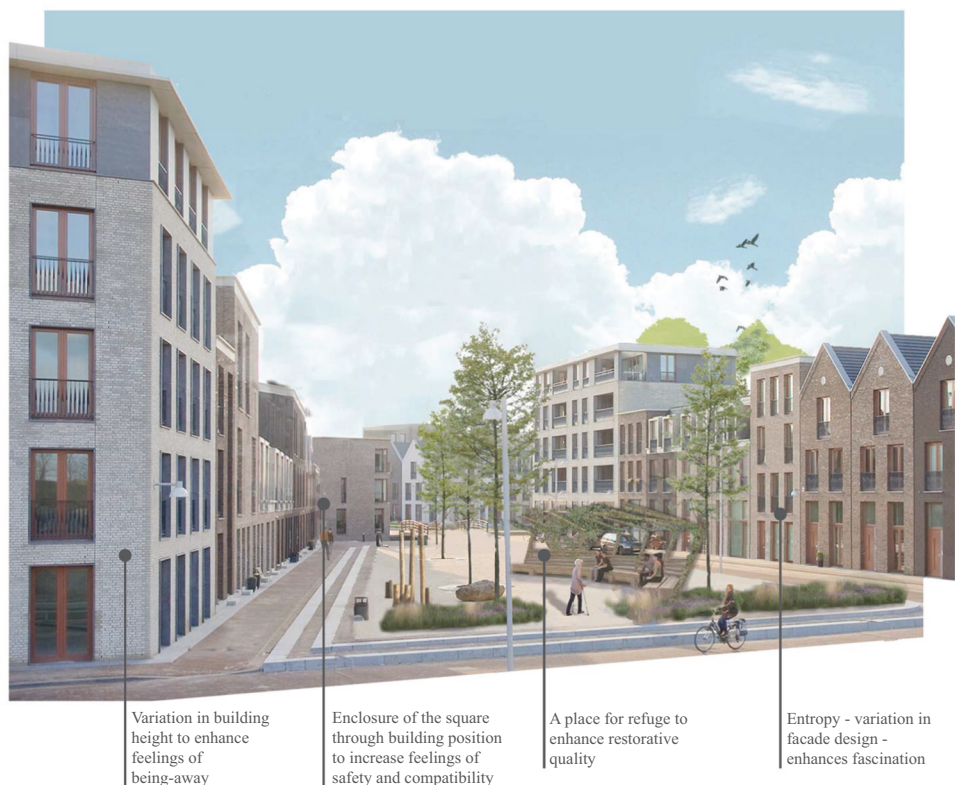
Figure 6. Impression of a restorative neighbourhood open space with architectural characteristics that enhance the environment's restorative quality. Image by the authors.
